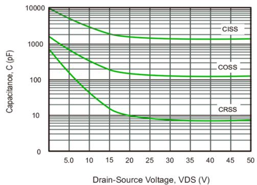
Fig.4 Capacitance Characteristics
